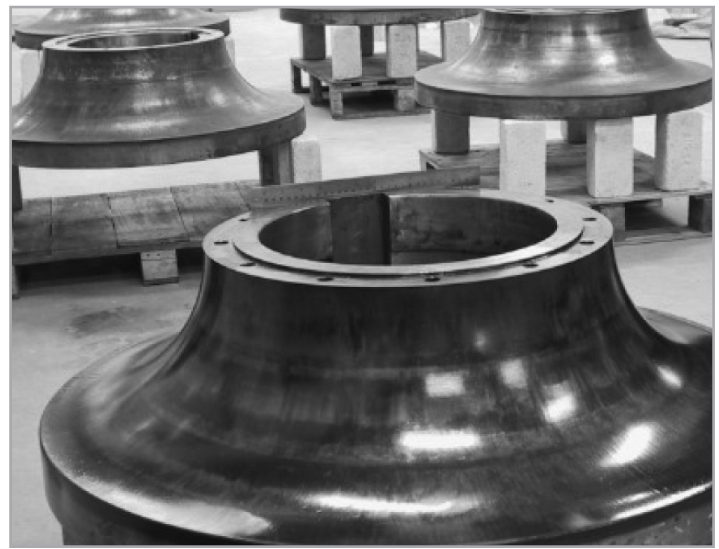
Figure 12: Induction Hardened Rollers
