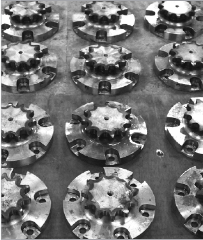
Figure 14a: Induction hardened sprocket gear hub
