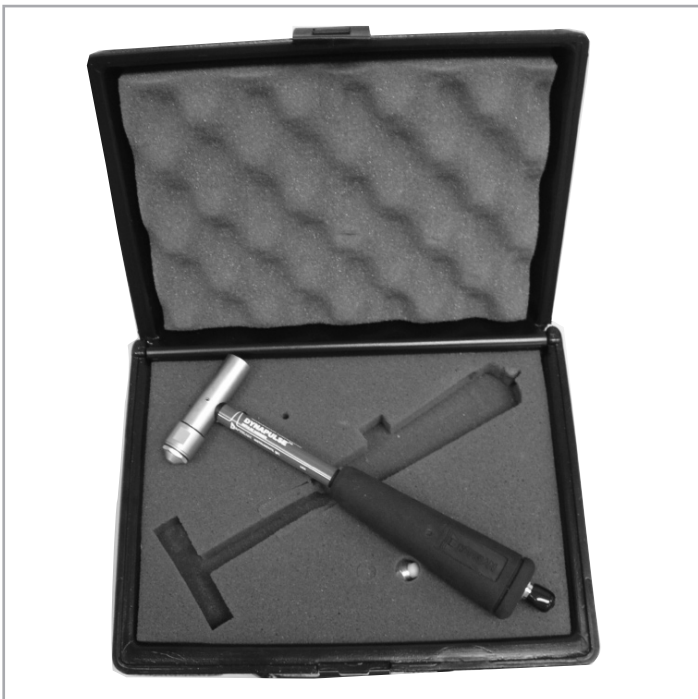
Figure 6: Instrumented hammer for the experimental modal analysis
