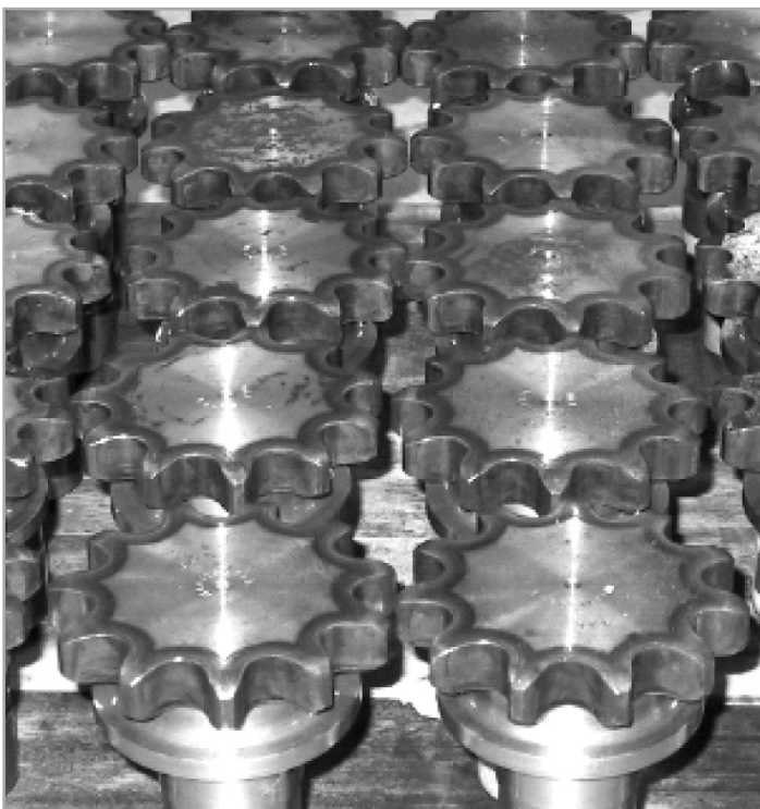
Figure 14b: Induction hardened sprocket gear shaft
