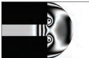
(v) Shock front position at x = 23.5 \text{ cm} , density fringes step 0.1
