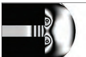
(vi) Shock front position at x = 28.5 \text{ cm} , density fringes step 0.1
