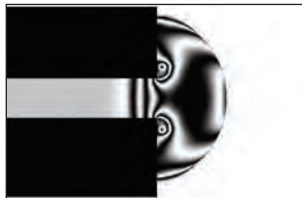
(iv) Shock front position at x = 18.5 \text{ cm} , density fringes step 0.1
