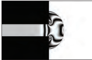
(iii) Shock front position at x = 13.75 \text{ cm} , density fringes step 0.1
