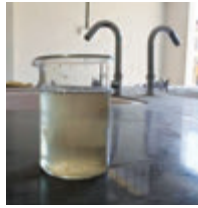
Figure 10: Effluent from UASB
