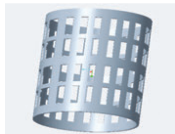
Figure 10: 3D View of filter vent in CREO
