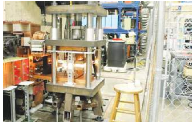
Figure 8: Experimental homopolar generator used in pulsed-welding applications. Reproduced from The potential of homopolar-generator welding (The Fabricator, 2019)
