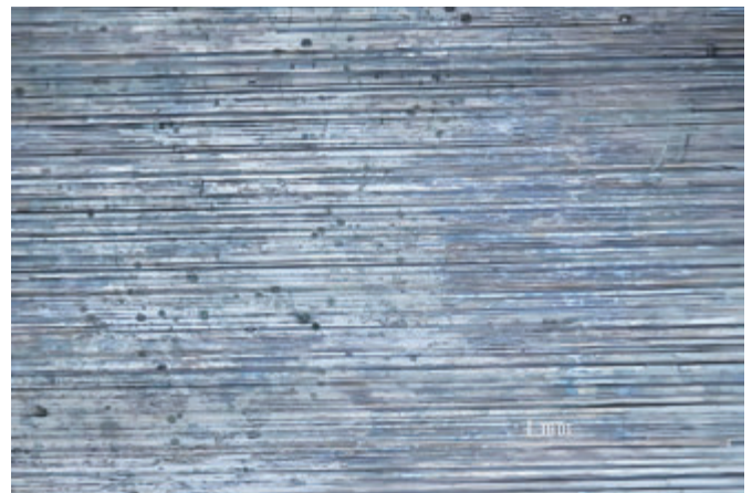
Figure 4: Diagram of Titanium alloy with lowest surface roughness using Tungsten Carbide insert
