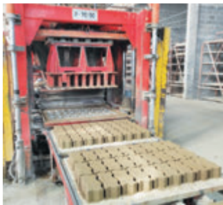
Figure 2: After demolding from machine mold
