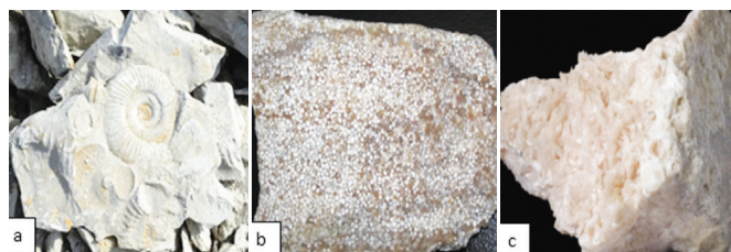
Figure 5 (a): fossiliferous limestone texture, (b): micritic limestone, (c): crystalline limestone texture Access online via https://geology.com
