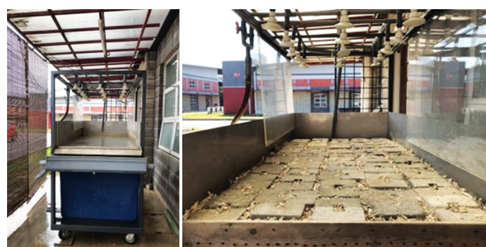
Figure 1: Lab Scale Simulation of Pavement Runoff using Rainfall Simulator System (RSS)
