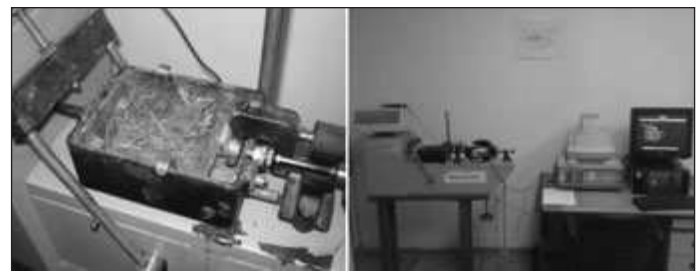
Figure 6: Soil Block Placed in the Shear Box
