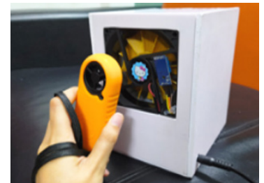
Figure 9: Airflow test setup Figure 10: Cooling rate test setup
