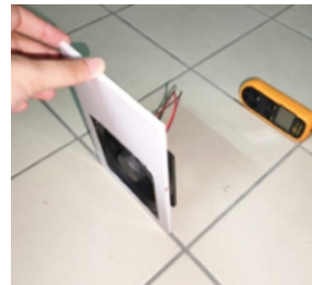
Figure 9: Airflow test setup Figure 10: Cooling rate test setup
