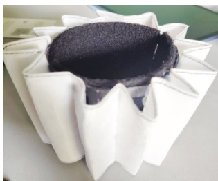
Figure 18: The combined filters which consists of thin and thick interlining fabrics (most outer side) and activated carbon filter (internal side)
