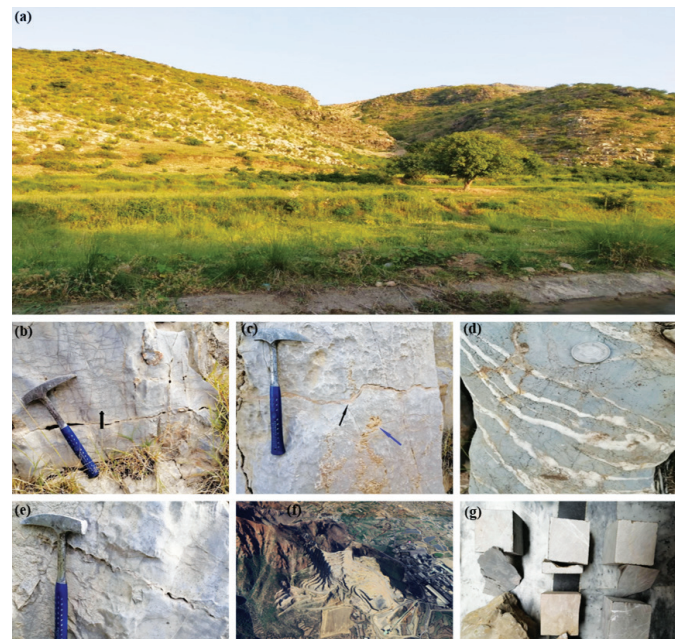
Figure 5: Geological features and strength testing of the Samana Suk Formation at Village Rani Wah, Hattar-Khanpur (a) Panoramic view of the exposed limestone beds; (b) Thick-bedded limestone with fractures (hammer for scale); (c) Medium-bedded limestone exhibiting bioturbation and dolomite-filled veins (hammer for scale); (d) Parallel calcite veins within the medium-bedded limestone (coin for scale); (e) Stylolite structures formed under compressive stress (hammer for scale); (f) Limestone quarry near the study area; (g) Cubes (4"x4"x4") used for Unconfined Compressive Strength (UCS) and Tensile Strength testing of limestone samples
