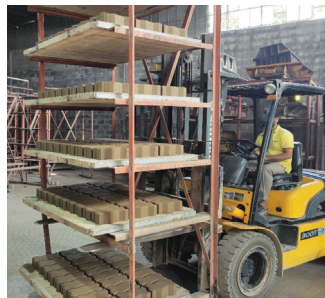
Figure 3: Carrying to the storage place for curing
